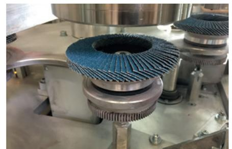
Manufacturing of flap discs as well as flap wheels
